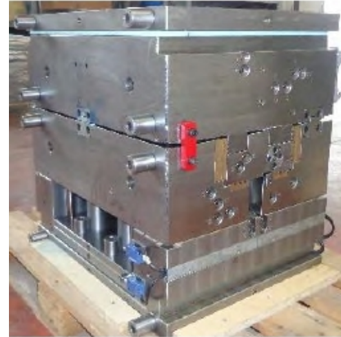
Mould steel hardened "Mostrina mobiletto"
